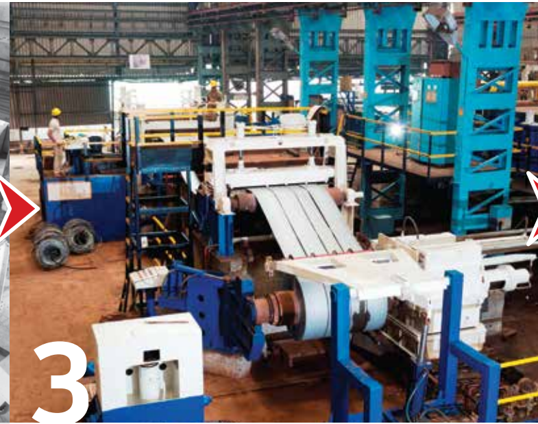
HR SLITTING Pickled coils are slit to desired width to prepare narrow strips for further processing • Slitting line capacity of 180,000 mt per annum • Can slit up to 6 mm thickness
