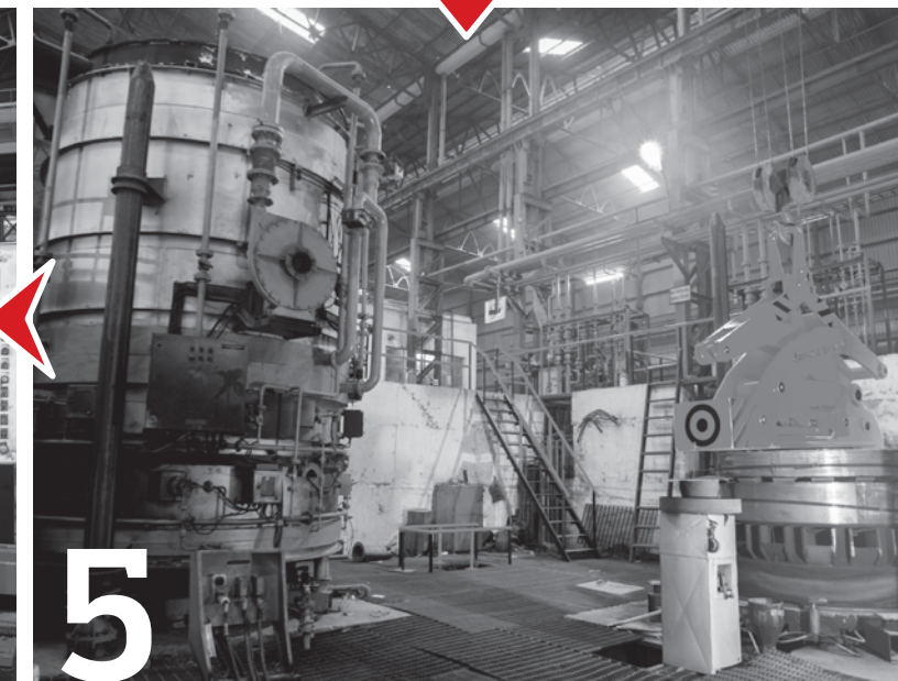
BELL ANNEALING FURNACE To remove strain and to obtain desired grain structure for improved mechanical properties, the strips are heated and control cooled in an inert atmosphere. • Hydrogen and nitrogen gases used as inert media • Superior surface cleanliness • Spherodisation/recrystallisation annealing • Mechanical properties as per IS standards
