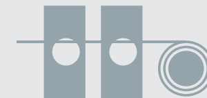
BELL ANNEALING FURNACE To remove strain and to obtain desired grain structure for improved mechanical properties, the strips are heated and control cooled in an inert atmosphere. • Hydrogen and nitrogen gases used as inert media • Superior surface cleanliness • Spherodisation/recrystallisation annealing • Mechanical properties as per IS standards
